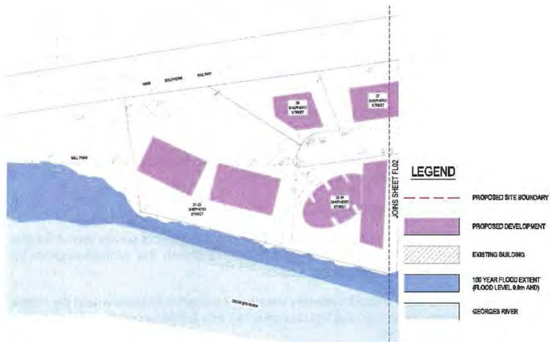
Figure 25. 100 Year Flood levels (southern section) Source: Wood & Grieve Engineers
